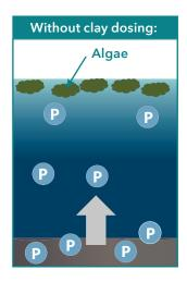
The hydrotalcite clay binds with phosphorus in the water making it unavailable to algae. It also forms a protective layer on the sediments preventing phosphorus release.
