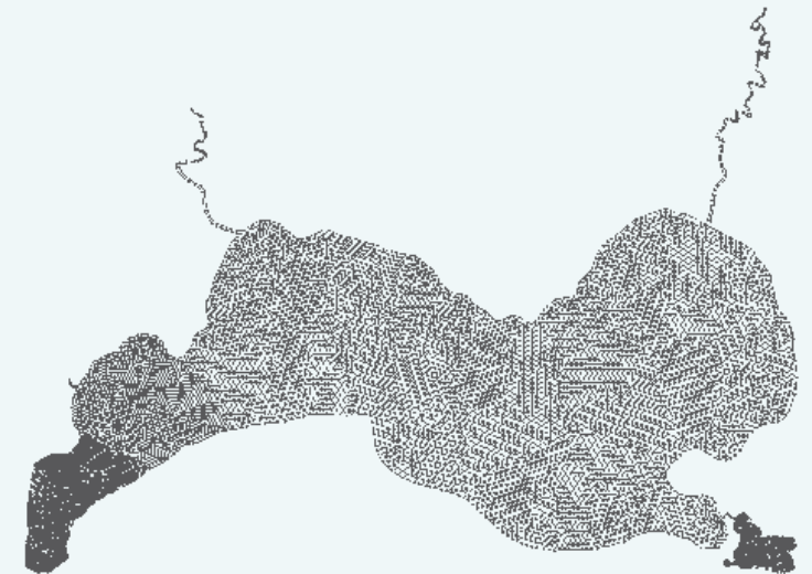
Wilson Inlet estuary model grid showing the individual cells where equations are resolved to determine water circulation and physical properties.
